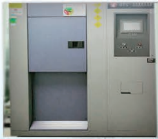
Hot And Cold Shock Test Room
