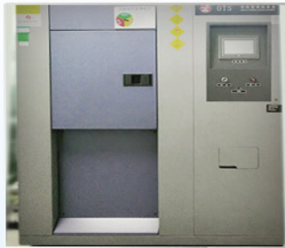
Hot And Cold Shock Test Room
