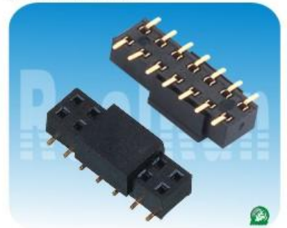
02.5 系列: 2.54mm双排母,SMT,U形端子 (可带定位柱及夹持盖) Spec:2.54mm Female Header,Dual Row, SMT With Locating Peg Or CAP Positions:2*2~2*40 Plastics Height:3.5mm
