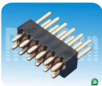
01.5系列: 2.54mm双排针,180度 Spec:2.54mm Pin Header,Dual Row,Straight Positions:2*3~2*40 Plastics Height:4.3mm
