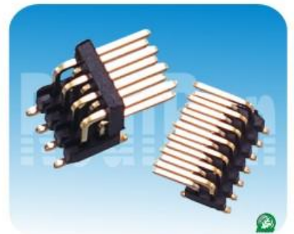
01.5系列:2.54mm排针 双排 90度 SMT 加塑胶 Spec:2.54mm Pin Header Dual Row Right Angle SMT Positions:2*2~2*50 Plastics Height:1.0/1.5/2.0/2.54mm
