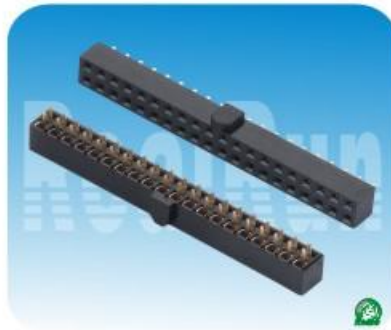
02.5 系列: 2.54mm双排母,180度带凸点,塑高5.0mm Spec:2.54mm Female Header,Dual Row, Straight With Polarizatic Positions:2*2~2*40 Plastics Height:5.0mm
