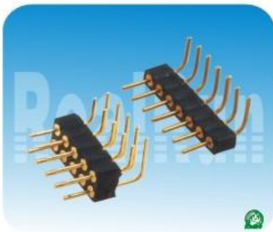
01.8系列:2.0mm 圆针 单/双排 90度 Spec:2.0mm Pitch Machine Pin Adapters Single/Dual Row Right Angle Plastics Height:2.8 Positions:1*2~1*40/2*2~2*40
