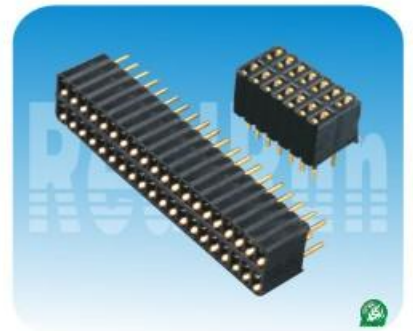
02.3系列: 1.27*2.54mm双排母,180度 Spec:1.27*2.54mm Female Header,Dual Row,Straight Positions:2*2~2*50 Plastics Height:4.6mm
