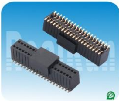
02.3系列: 1.27*2.54mm双排母,SMT (可带定位柱及夹持盖) Spec:1.27*2.54mm Female Header,Dual Row, SMT With Locating Peg or CAP Positions:2*2~2*50 Plastics Height:5.7mm
