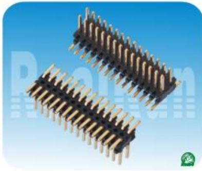
01.1系列: 0.8*1.2mm双排针 贴片 Spec:0.8*1.2mm Pin Header,Dual Row,SMT Positions:2*2~2*50 Plastics Height:1.38mm
