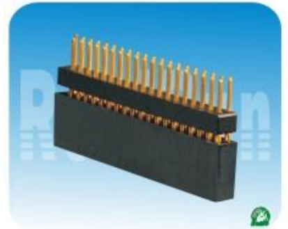
02.5系列: 2.54mm双排母,180度,PC104 免焊接式 Spec:2.54mm Female Header,Dual Row, Straight Press-Fit Positions:2*2~2*40P Plastics Height:11.0mm
