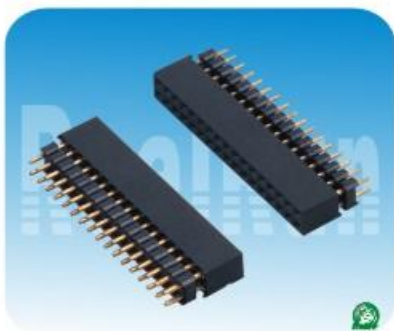
02.4系列: 2.0mm双排母,180度 Spec:2.0mm Female Header,Dual Row,Straight Positions:2*2~2*40 Plastics Height:6.35+2.0mm
