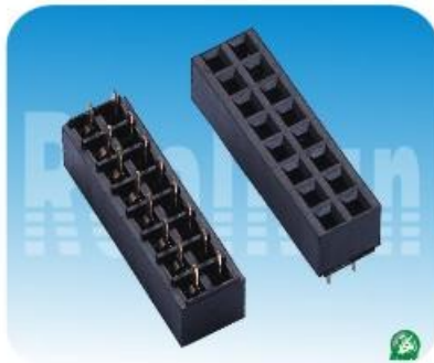
02.5系列: 2.54mm单/双排母,180度,塑高6.8mm下插型 Spec:2.54mm Female Header,Single Dual Row, Bottom Entry ,Straight Positions:1*2~1*40/2*2~2*40 Plastics Height:6.8mm
