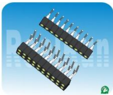
02.A系列:2.0mm 圆孔 单/双排 90度 Spec:2.0mm Pitch Machine Pin Socket Single/Dual Row Right Angle Plastics Height:2.8 Positions:1*2~1*40/2*2~2*40
