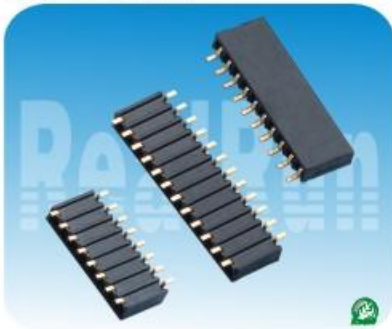
02.5 系列: 2.54mm单排母,SMT,侧插型 Spec:2.54mm Female Header,Single Row, Side Entry SMT Positions:1*2~1*40 Plastics Height:3.4mm
