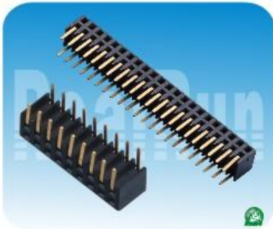
02.4 系列: 2.0mm双排母,90度,侧插型 Spec:2.0mm Female Header,Dual Row, Side Entry,Right Angle Positions:2*2~2*40 Plastics Height:4.9mm
