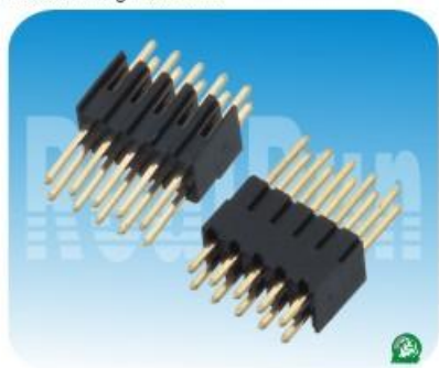
01.5系列: 2.54mm双排针,180度 Spec:2.54mm Pin Header,Dual Row,Straight Positions:2*3~2*40 Plastics Height:7.4mm
