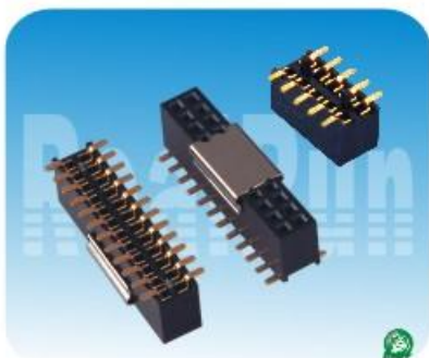
02.3系列: 1.27mm双排母,SMT,(可带定位柱及夹持盖) Spec:1.27mm Female Header,Dual Row, SMT With Locating Peg or CAP Positions:2*2~2*50 Plastics Height:2.0/3.4/4.3mm
