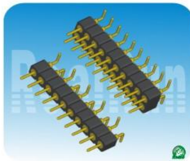
01.8系列:2.0mm 圆针 单/双排 SMT Spec:2.0mm Pitch Machine Pin Adapters Single/Dual Row SMT Plastics Height:2.8 Positions:1*2~1*40/2*2~2*40
