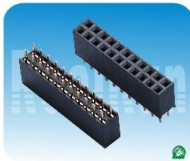
02.5系列: 2.54mm双排母,180度,Y形端子 Spec:2.54mm Female Header,Dual Row,Straight Positions:2*2~2*40 Plastics Height:5.7/8.5mm Y-Type Terminal
