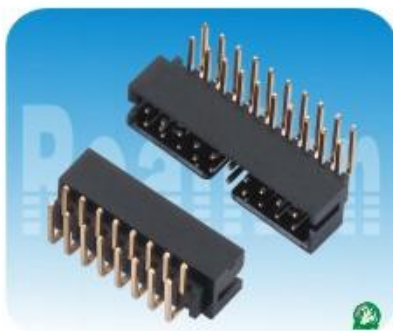
03.4系列: 2.0mm简易牛角,90度 Spec:2.0mm Box Header,Right Angle Positions:10-80 Plastics Height:6.4mm
