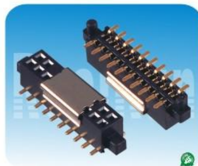
02.3系列: 1.27mm双排母,SMT (带大小定位柱及夹持盖) Spec:1.27mm Female Header,Dual Row, SMT With Different Locating Peg or CAP Positions:2*2~2*50 Plastics Height:3.4mm
