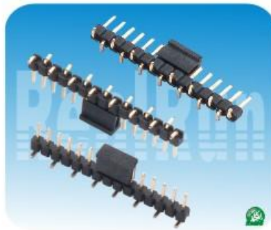
01.4 系列: 2.0mm单排针,180度,SMT,(可带夹持盖) Spec:2.0mm Pin Header,Single Row,SMT With CAP Positions:1*3~1*40 Plastics Height:1.0/1.5/2.0mm
