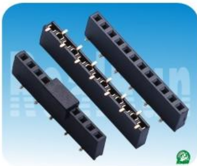
02.5系列: 2.54mm单排母,SMT,U形端子 (可带夹持盖) Spec:2.54mm Female Header,Single Row,SMT With CAP Positions:1*3~1*40 Plastics Height:7.1/8.5mm
