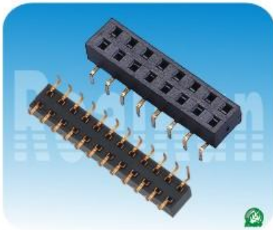
02.5 系列: 2.54mm双排母,蜈蚣脚,U形端子 Spec:2.54mm Female Header,Dual Row,Botton Entry Positions:2*2~2*40 Plastics Height:3.5mm
