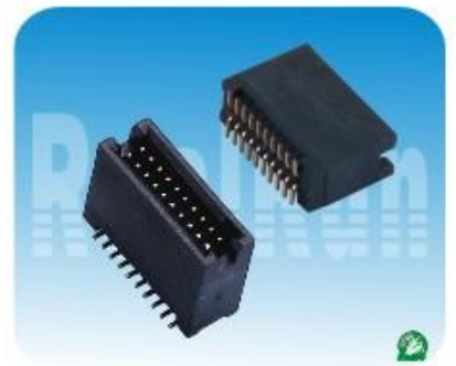
03.3系列: 1.27mm筒牛,SMT,加高型塑高 Spec:1.27mm Box Header,SMT,Elevator Positions:10~100 Plastics Height:7.5/8.0/9.0/10.0/12.0/15.0mm
