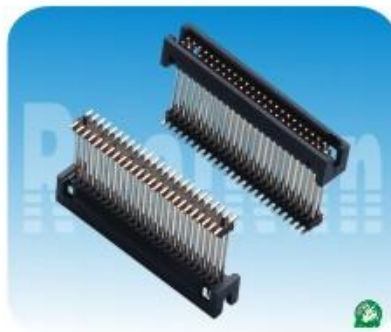
03.3系列: 1.27mm筒牛加塑胶,SMT Spec:1.27mm Box Header,SMT,Elevator Positions:10~100 Plastics Height:5.7mm
