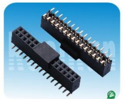
02.5系列: 2.54mm Female Header Dual Row,S.M.T Positions:2*2~2*40 Plastics Height:5.7/8.5mm Y-Type Terminal
