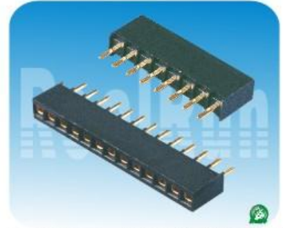
02.5系列: 2.54mm单排母,180度,塑高6.8mm上插型 Spec:2.54mm Female Header,Single Row,Top Entry, Straight Positions:1*2~1*40 Plastics Height:6.8mm
