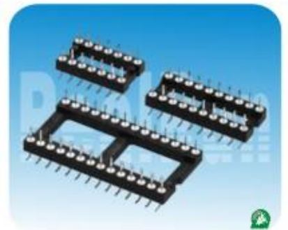
30.3系列:2.54mm 圆针 IC座 SMT H3.0 Spec:2.54mm Pitch Machine Pin IC Adapters SMT H3.0 Positions:A Type6/8/10/14/16/18/20/22/24/28 B Type20/22/24/28/32 C Type24/28/32/36/40/42/48
