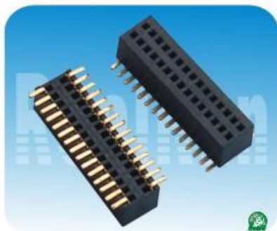
02.1系列: 0.8*1.2mm双排母,SMT Spec:0.8*1.2mm Female Header,Dual Row,SMT Positions:2*2~2*50 Plastics Height:3.1mm
