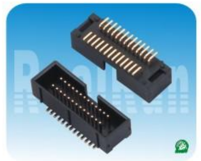
03.3系列: 1.27*2.54mm筒易牛角,SMT Spec:1.27*2.54mm Box Header,SMT Positions:10~100 Plastics Height:5.6mm
