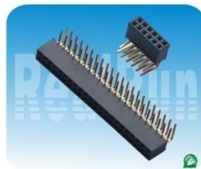
02.4系列: 2.0mm双排母,90度 Spec:2.0mm Female Header,Dual Row,Right Angle Positions:2*2~2*40 Plastics Height:6.35mm
