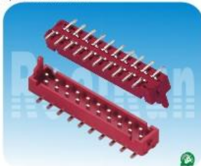
05.3系列：红色IDC CONNECTORS SERIES 1.27mm Micro Connectors Dual Row Male Contact. No.Of Contact:4 Through 26Pin Termination Styles: Surface Mounting Type. Tail Pitch:2.54mm. Spec:Without Latch.
