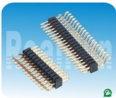
01.3系列: 1.27mm双排针,90度,SMT (可带定位柱及夹持盖) Spec:1.27mm Pin Header,Dual Row,Right Angle,SMT With Locating Peg Or CAP Positions:2*2~2*50 Plastics Height:2.0/2.54mm
