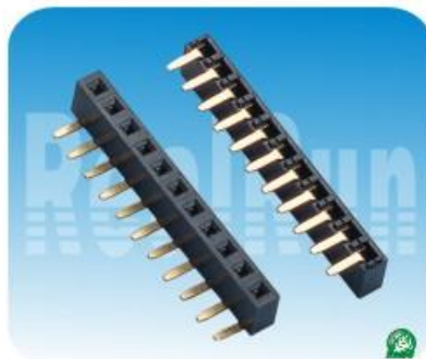
02.5 系列: 2.54mm单排母,90度,塑高5.0mm Spec:2.54mm Female Header,Single Row,Right Angle Positions:1*2~1*40 Plastics Height:5.0mm
