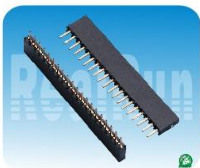
02.4系列: 2.0mm单排母,180度 Spec:2.0mm Female Header,Single Row,Straight Positions:1*2~1*40 Plastics Height:6.35mm
