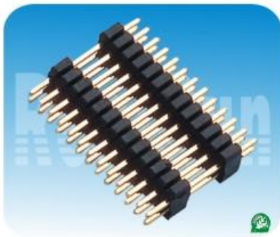
01.2系列: 1.0mm双排针,双塑,180度 Spec:1.0mm Board Spacer,Dual Row,Straight Positions:2*2~2*50 Plastics Height:1.0/1.5/2.0mm
