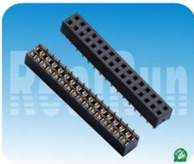
02.4系列: 2.0mm双排母,180度 Spec:2.0mm Female Header,Dual Row,Straight Positions:2*2~2*40 Plastics Height:2.2/4.0/4.3/4.6mm
