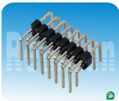
01.3系列: 1.27mm排针 双排 U型 Spec:1.27mm Pin Header Dual Row U type Plastics Height:1.0/1.5/1.7/2.0/2.54mm Positions:2*2~2*50
