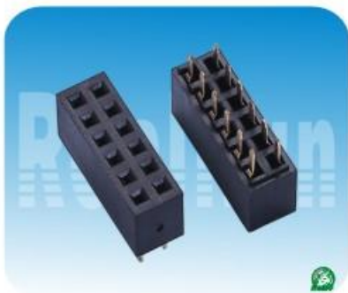
02.5系列: 2.54mm双排母,180度,U形端子 Spec:2.54mm Female Header,Dual Row,Straight Positions:2*2~2*40 Plastics Height:8.5mm U-Type Terminal
