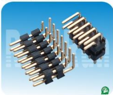
01.5系列: 2.54mm双排针,双塑,90度 Spec:2.54mm Board Spacer,Dual Row,Right Angle Positions:2*2~2*40 Plastics Height:2.54mm
